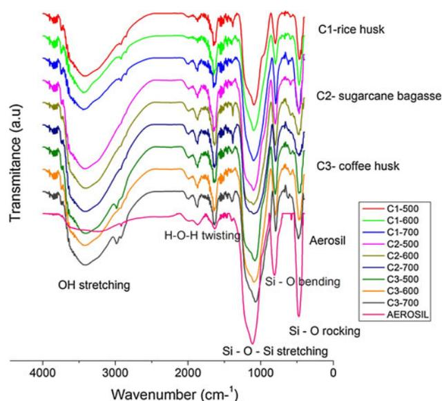
**Fig. 1** IR bands to synthesis of nanoparticles  $\text{SiO}_2$  obtained for vermicompost. The Figure show the bands more representatives to  $\text{SiO}_2$  to in rice husk, sugarcane bagasse and coffee husk at temperature of calcination: 500, 600 and 700°C. Representative bands for Aerosil® 130 too are shown
