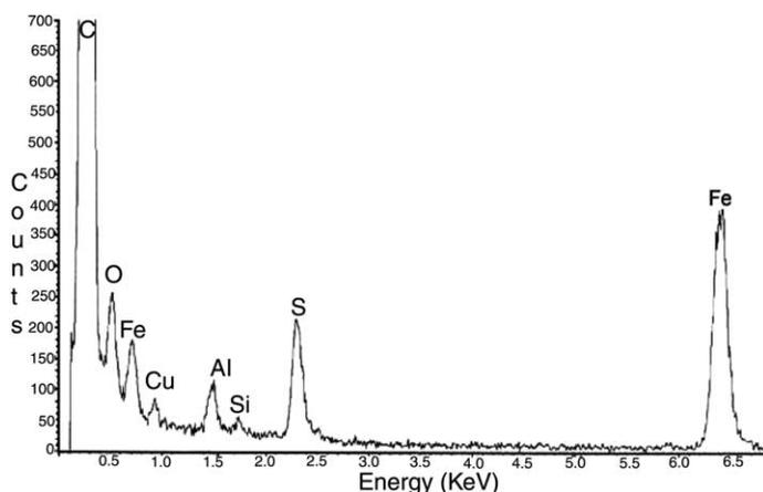
Fig. 2. EDS spectrum of natural carbon nanotubes.
