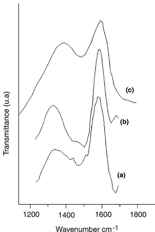
Fig. 3. First-order RAMAN spectra: (a) natural carbon nanotubes; (b) multiwalled carbon nanotubes arc discharge approach; (c) multiwalled carbon nanotubes produced at low temperature (reproduced with the author's permission) [18].
