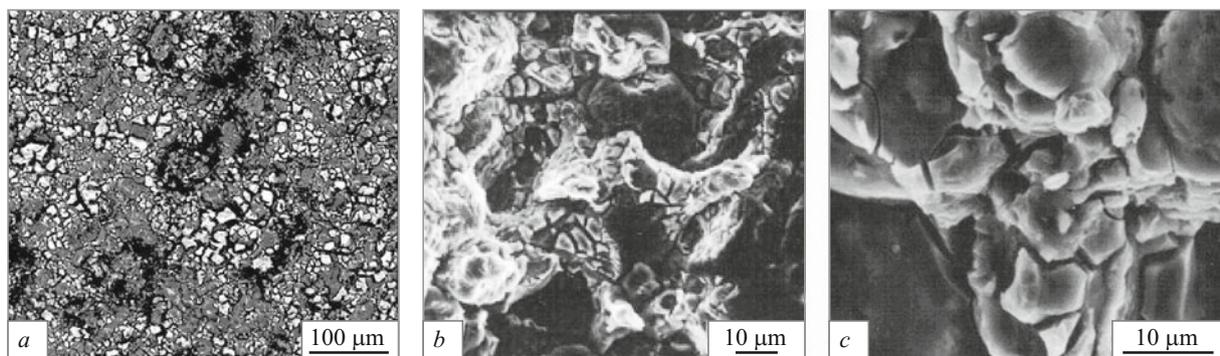
Fig. 3. SEM Micrograph of aluminum – zirconia composite.
