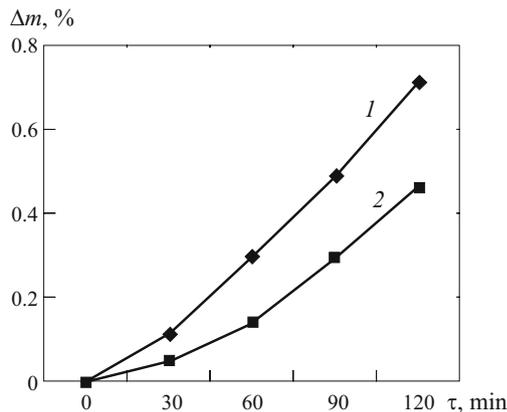
Fig. 2. Wear vs. time for aluminum – zirconia composites and pure aluminum.
