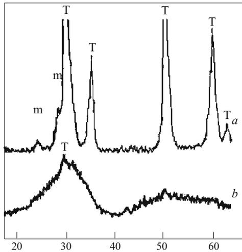
Fig. 1. XRD diffractogram of zirconia after sintering.
