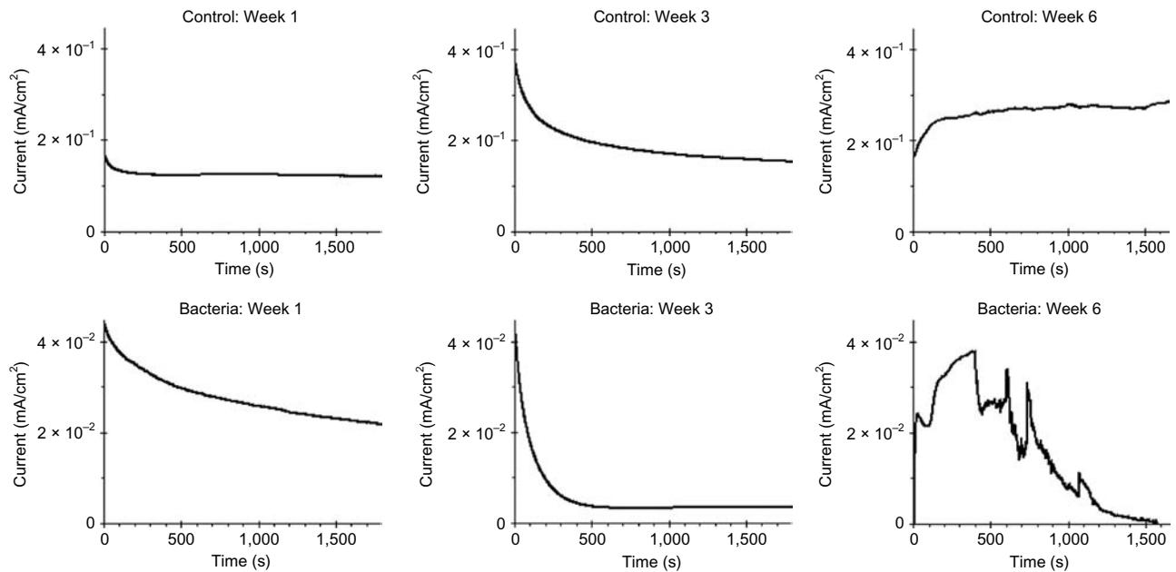
**Figure 2** Potential EN of copper electrodes isolated, control samples (upper) and under bacteria strain (lower) in weeks 1, 3, and 6
