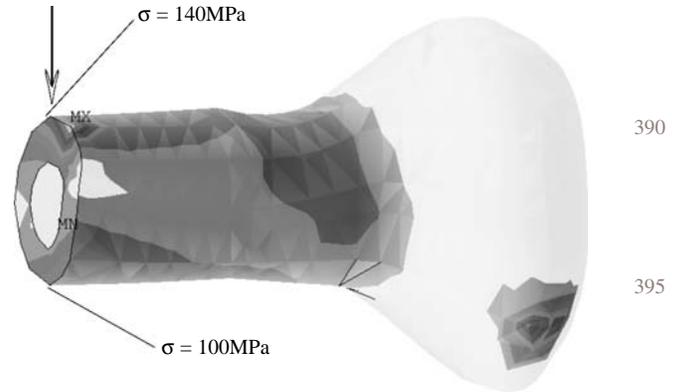
Figure 6. von-Misses stresses for  $P = 1000$  kg.
