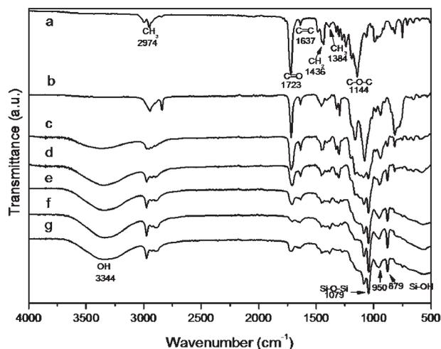
a PMMA; b 3-(trimethoxysilyl)propyl methacrylate; c 90-10; d 75-25; e 50-50; f 25-75; g 10-90
