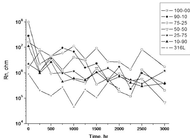
**7** Noise resistance  $R_n$  as function of exposure time in 5 wt-% NaCl solution
