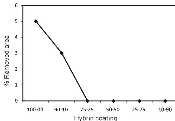
6 Measuring adhesion by tape test on PMMA-silica hybrid sol-gel coatings according to ASTM D3350
