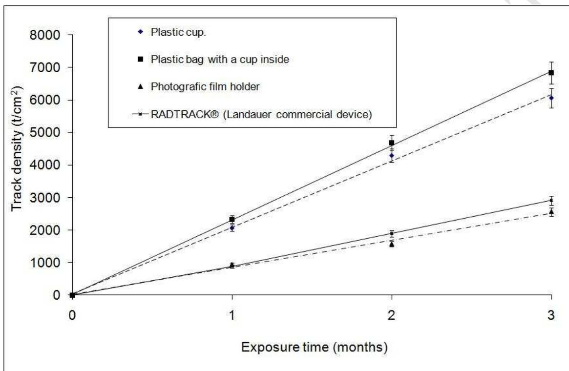
Figure 3.- Response of the different devices as function of exposure time.
